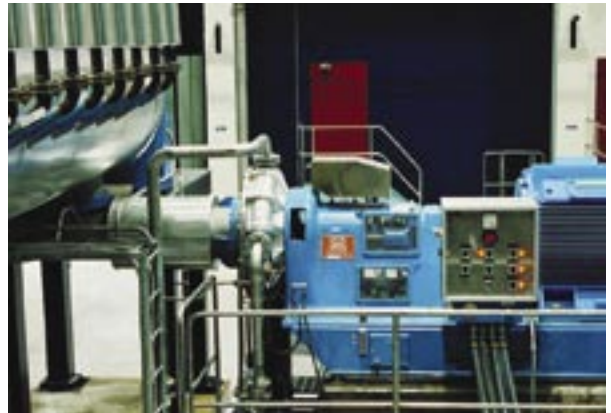
Disc refiner with SK 700 tracer valve
