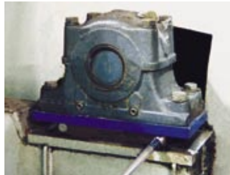
Web tension measurement unit in dryer section
