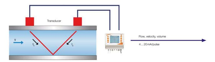
**Mounting in Z-mode** (applicable for big pipe dimensions or high acoustic damping)
